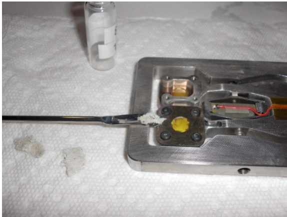
Figure one: Asbestos insulation sample
